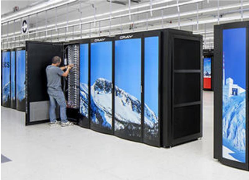
With “Piz Daint,” the Swiss National Supercomputing Centre (CSCS) is putting a new supercomputer system in operation that will provide necessary compute performance and consume less power. This is made possible by a novel hybrid computer system which makes use of sophisticated graphics processors (GPUs) as used in the gaming industry.
