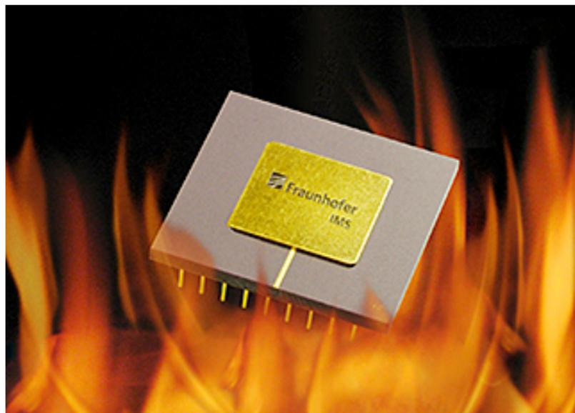
*Temperatures often over 200 degrees C occur in geothermal and oil production — conventional microelectronics hit their limits there. Researchers have now fabricated compact microchips that can keep their cool even at 300 degrees C.*
