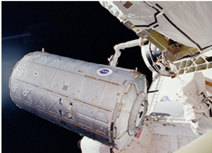
[1]On February 10, 2001, the crews of the Space Shuttle Atlantis and the International Space Station successfully installed the U.S. Destiny Laboratory onto the station. In this photo, Destiny is moved by the shuttle's remote manipulator system (RMS) robot arm from its stowage position in the cargo bay of the Space Shuttle Atlantis.
